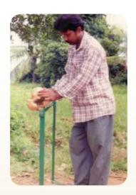
a portion of the husk. The operation is repeated 3-4 times until complete de-husking is done.
