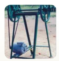
ments for shelling maize cob / threshing sunflower ear-heads. A shaft driven by an electric motor rotates at about 200 rpm. On both ends of the shaft, either the maize shelling (tubular sheller) or sunflower threshing attachments (disc with pins) are fixed. Individual cob / ear-head is shelled / threshed manually and the seed damage is bare minimum making it suitable for seed production.
