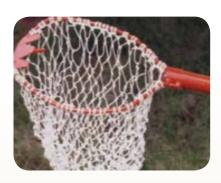
cutting the petiole of the fruit. Nylon net is fixed to the metal ring to hold the plucked fruits. The unit needs to be fixed to a long pole of suitable length to reach the fruits on the tree.
