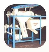
power operated green pea pod sheller to meet the requirement of the pea growers. The sheller consisted of feeding hopper, roller, concave, frame and a 0.25 hp electric motor. The roller is fixed on a central shaft supported on two bearings. The roller rotates in the concave. The roller and concave assembly are mounted on a frame. The concave consists of galvanized iron sheet punched with holes of 16mm dia. at a centre to centre distance of 26 mm.
